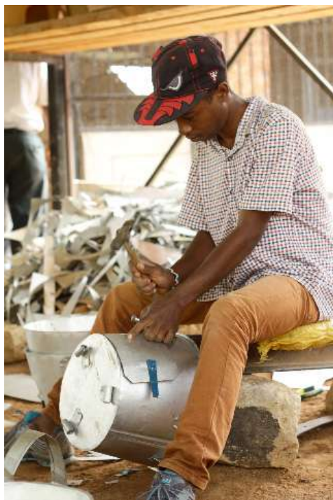
Institutional stove and a Stove technician fabricating a stove
